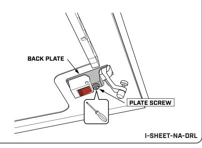
IF THIS DOES NOT FIX THE ISSUE, REMOVE THE SCREW AND BACK COVER PLATE USING A PHILLIPS HEAD SCREWDRIVER AS SHOWN.
