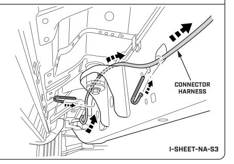
ROUTE THE CONNECTOR HARNESS UP AND OVER THE REAR WHEEL WELL.
