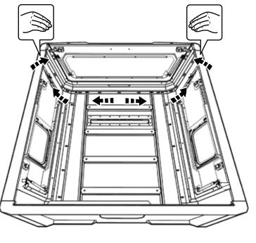
TIGHTEN ALL HARDWARE WITH TORQUE WRENCH AND 10MM SOCKET TO 3.7 FT. LBS. (5 NEWTON METERS)
