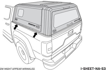
\*YOU MAY NOTICE THAT THE SEAL ON THE SLIDING PORTAL WINDOW MIGHT APPEAR WRINKLED. THIS IS DUE TO THE ANTI-SLIP COATING AND IS NOT A CAUSE FOR CONCERN.
