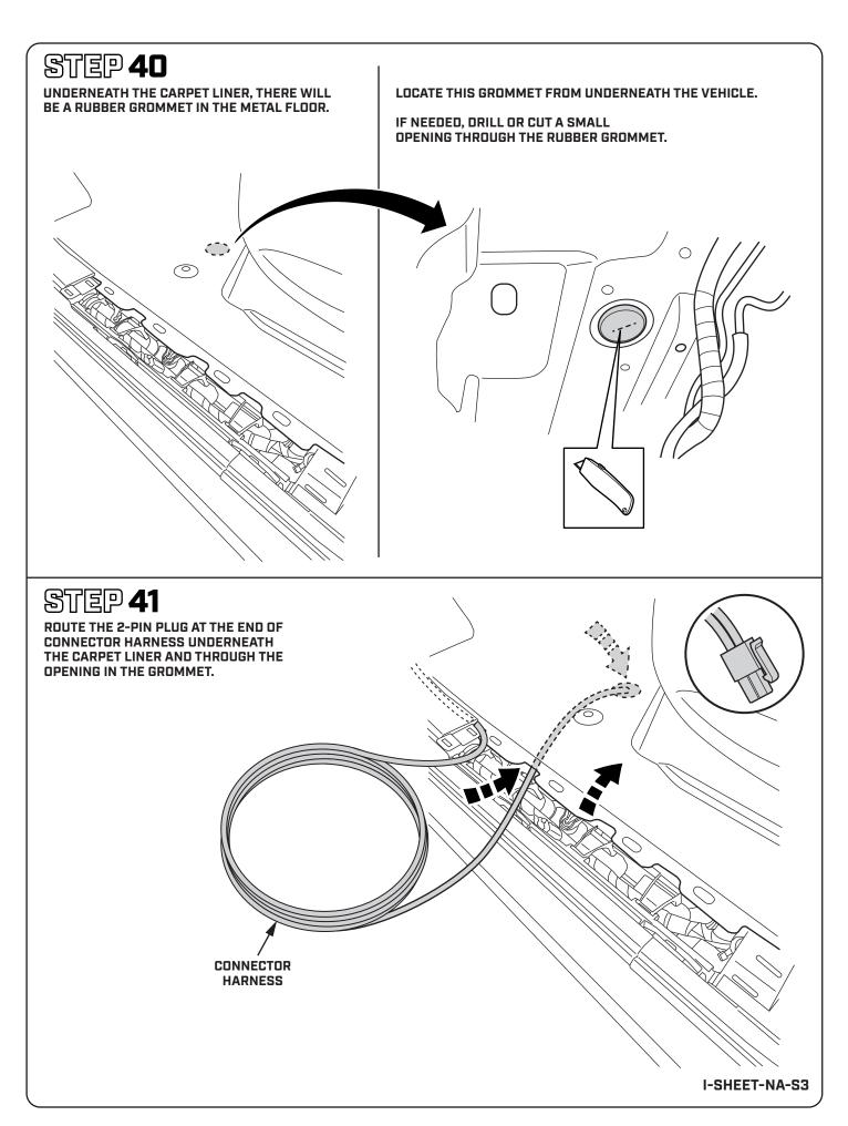
CAREFULLY PULL THE ENTIRE LENGTH OF THE CONNECTOR HARNESS DOWN THROUGH THE GROMMET.
