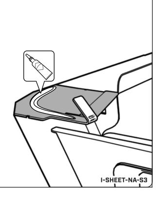
**FULLY INSERT THE RETENTION TAB** INTO THE SLOT ON THE D-RUBBER. **ENSURE THE D-RUBBER IS ORIENTED CORRECTLY WITH ITS PROFILE MATCHING** THE CONTOUR OF THE REAR FLANGE.
