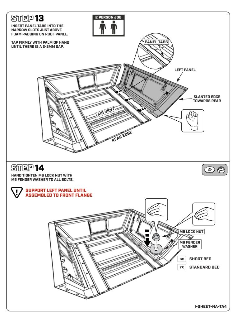
INSTALL HARDWARE ALONG FRONT FLANGE WITH BOLT ON INSIDE.
