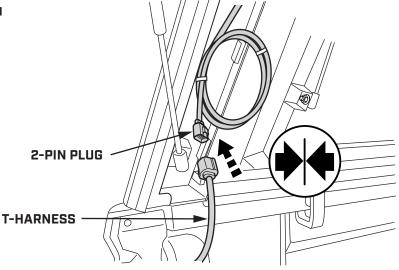
REMOVE THE GROMMET COVER AT THE TRUCK BED WALL.
